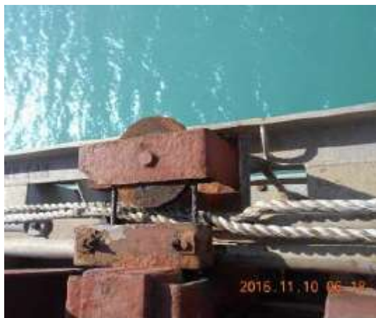
The sheave assembly where the wire jammed
